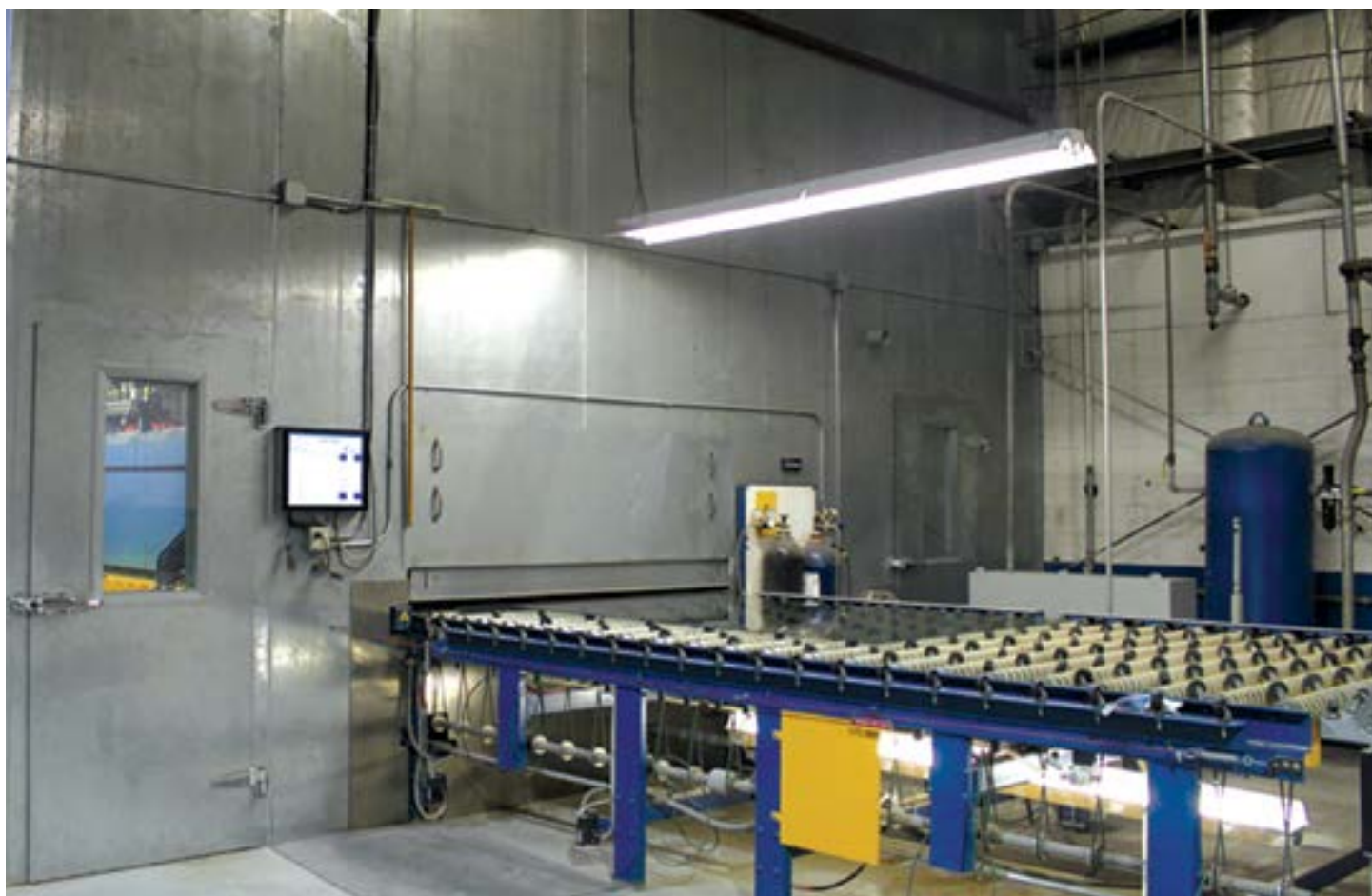
Rollers feed the glass into the tempering oven. Also referred to as "safety glass," tempered glass, shatters into small cubes when broken, as opposed to jagged shards.
